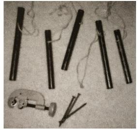
remove any sharp edge left on the pipe. Ream both the inside and outside diameters of both ends of the pipe chime. Then, drill a hole through each pipe chime at the node point and pass a string through these holes. Hold each pipe by this string loop and strike with a spoon or nail to produce a tone.
